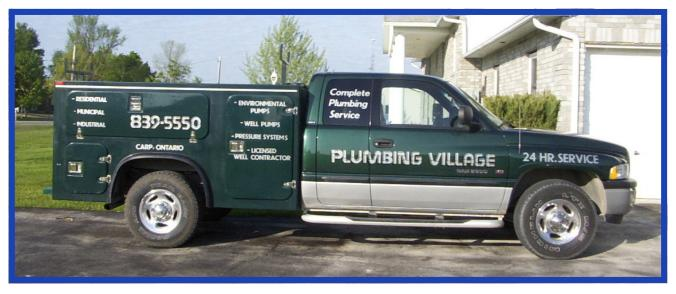
The BR98-48 truck body is ideal for small trucks. The lightweight fiberglass construction allows for more cargo carrying capacity. This truck body weighs in at 250 –300 pounds, not including the floor panel. The double-skinned doors make for a very lightweight, sturdy door.
